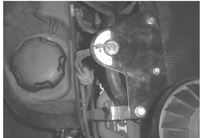
Left Tank: Fuel flows from the left tank when the selector is turned 1/4 turn toward the left hand side of the machine.
